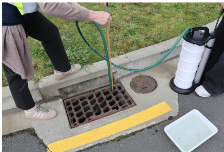
Figure 8. Attach a dowel to the hose to increase manoeuvrability
