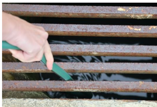
Figure 2. Using a fluid extractor to sample different types of sumps
