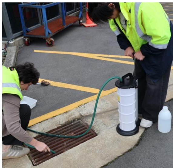
Figure 4. Two persons team sampling a sump using a fluid extractor
