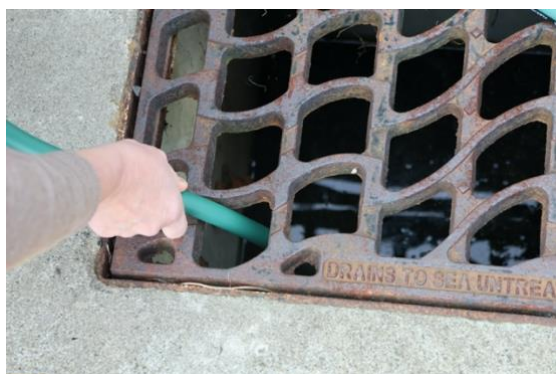
Figure 2. Using a fluid extractor to sample different types of sumps
