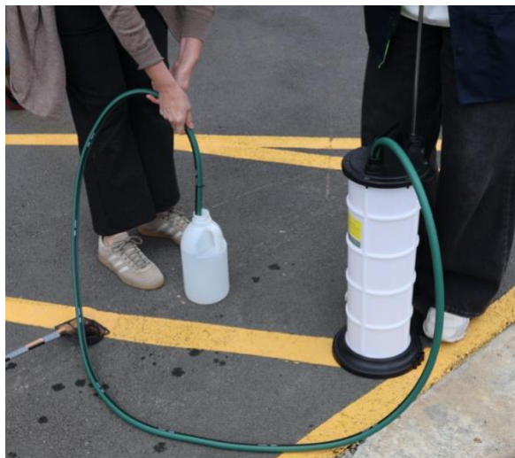
Figure 6. Pumping clean water in the fluid extractor
